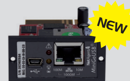
ZGR 310392 - MINI PRO SNMP card, Modbus TCP Compatibility: TOWER PRO / EFFICIENT RT VERSATILE / INFLUENCE
